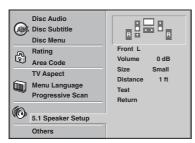
Select "5.1 Speaker Setup" using the ▲/▼ buttons on the setup menu.
